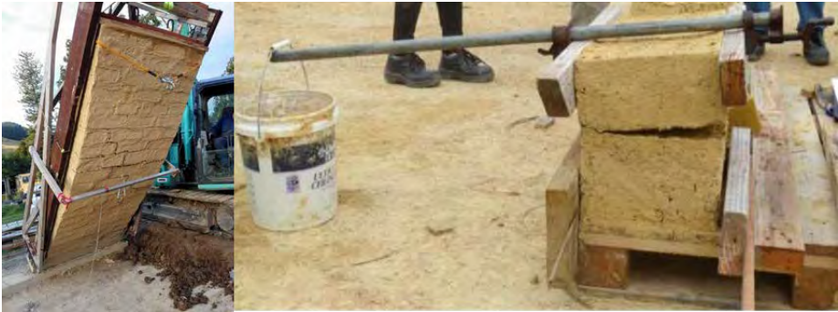
Figure 3: a) Lightweight adobe 230mm thick out-of-plane tilt test, b) Bond wrench test measuring mortar adhesion. Photos: Hugh Morris
