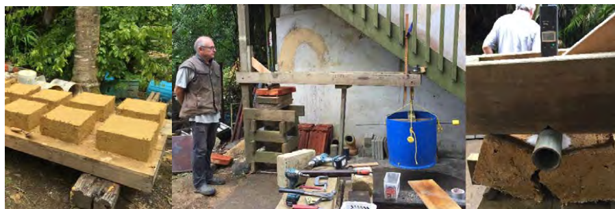
Figure 4. a) Low density adobe bricks b) Simple lever arm test setup using measured water for mass) c) detail of the load point after a flexural tension failure, Auckland 2019 Photos: Min Hall
