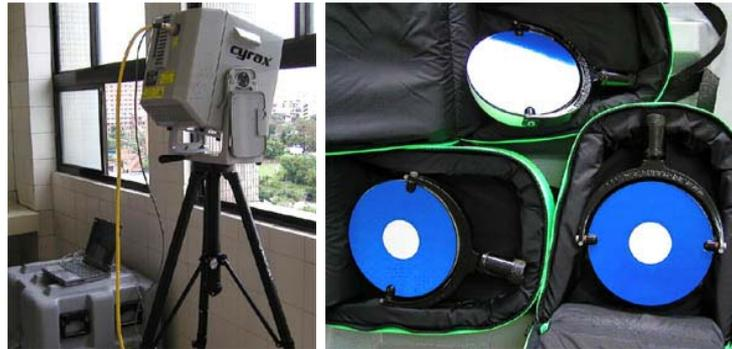
Figure 1: 3D scanner (left) and registration targets (right)
