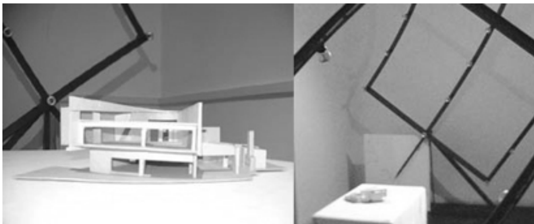
Figure 3: Our students are currently trained to carry out sunshine-path studies on models using a heliodon . However, this means is sometimes used just to obtain an impressive image of a blind-to-solar-orientation project.
